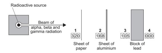
Match the radiation detected, A, B, C and D, with the positions 1–4 in the diagram.
